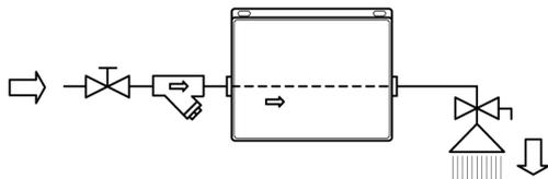
OSCAR II° plus, as opposed to normal water meters, may be wall-mounted, thus it is necessary to carry out the following operations in the set order:
